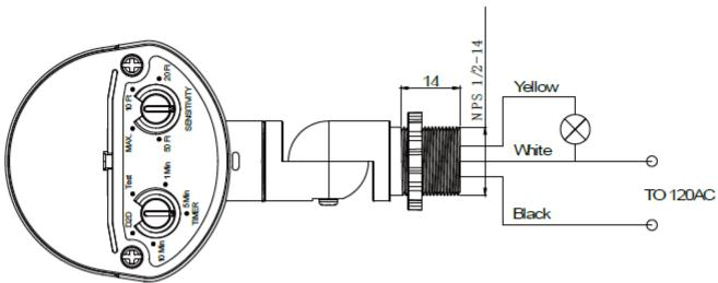
Wires in 1007 18AWG 80°C 300V
